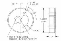
Precision side locator that can be doweled in place after adjustment. Use for vertical leveling or horizontal locating. Available hardened, or soft to allow drilling and reaming after installation.
