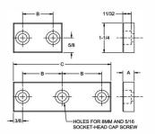
Large, precision rest pad for virtually any application. Peerless Rest Pads are extremely useful as supports, side locator pads, wear pads, or jig feet. Available both ground and unground for accurate height location. Mount with socket-head cap screws (not furnished).
